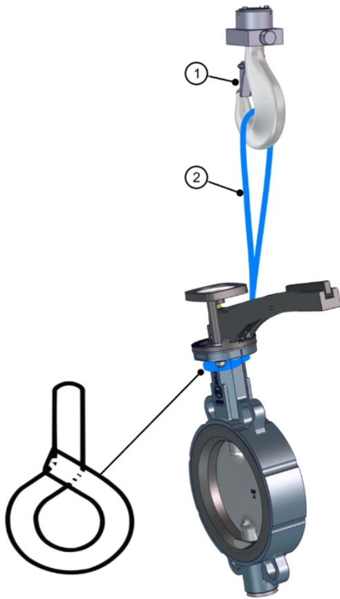
Fig. 6: Lifting wafer-type butterfly valve with a crane
