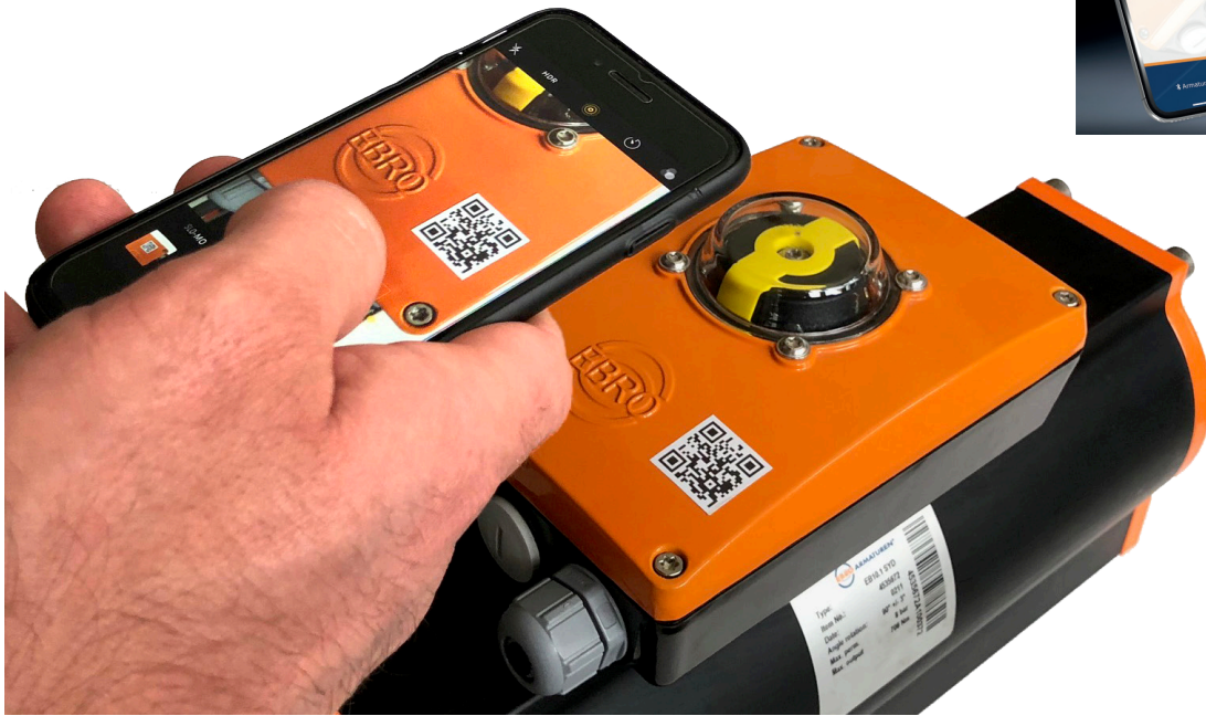
Fig 2: The app identifies the assembly via Bluetooth or QR code. Specifications and evaluations can be read out in plain text and transferred directly to the user's cloud.
