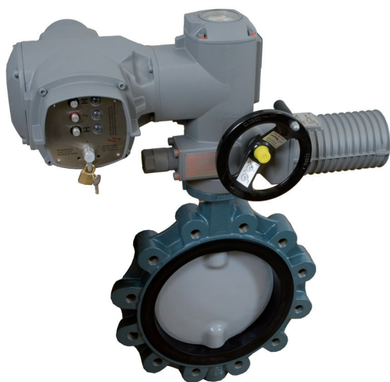
Fig. 2: butterfly valve with a UHMWPE lined disc and electric drive
