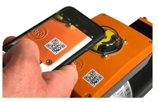
Figure 2: The app identifies the assembly via Bluetooth or a QR code. Specifications and analyses can be read in plain text and transmitted directly to the user's cloud.
