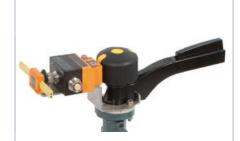
The AS-i bus connection for manual operated valves is achieved by a double sensor equipped with a flat cable connector and two inductive sensors. A puk indicates the valve position.
