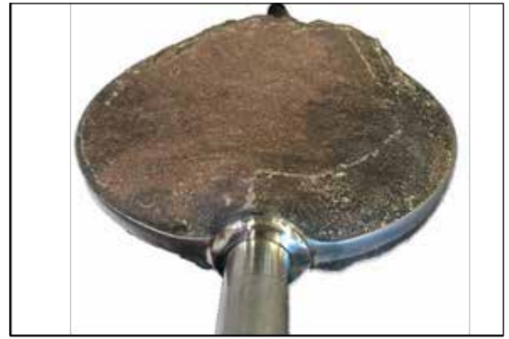
Figure 1: Worn conventional shut-off valve that no longer seals gas-tight
