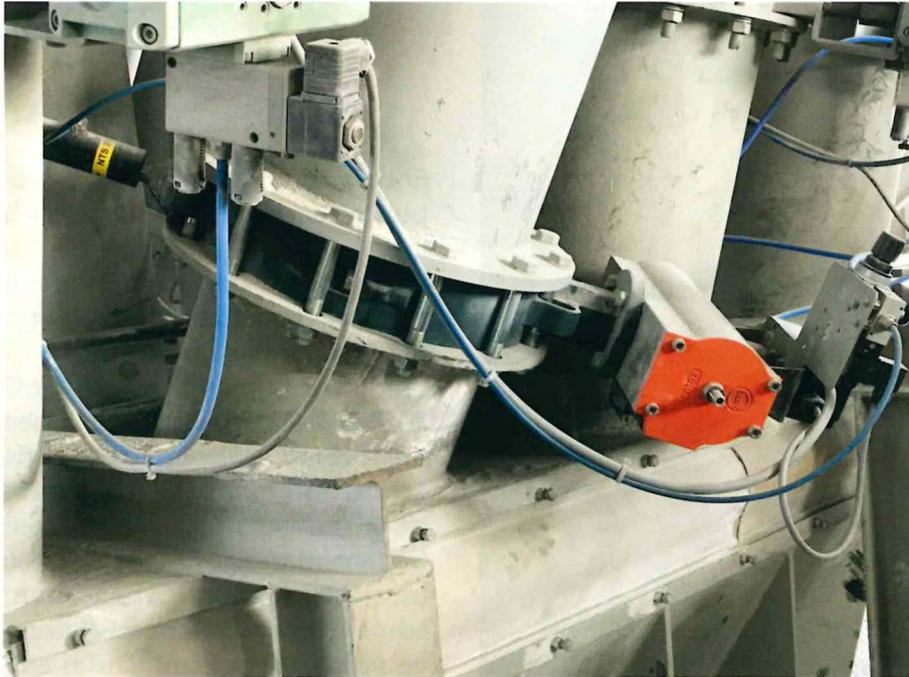
**Figure 2: ViDos® dosing valve for coarse/fine flow dosing of solids**
